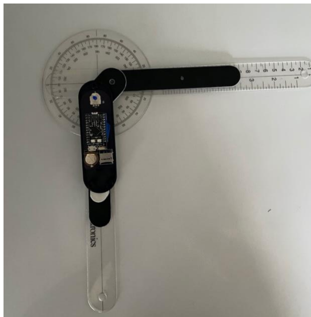
Figure 29. Device overlaid on goniometer bent at 90^\circ
