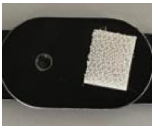
Figure 26a. The velcro on the axis of the hinge system that connects to the velcro on the rotor shaft
