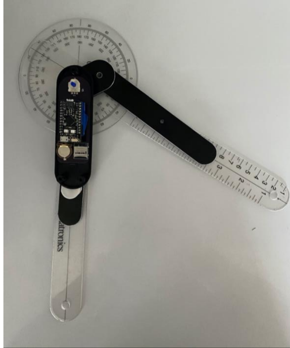
Figure 30. Device overlaid on goniometer bent at 120°
