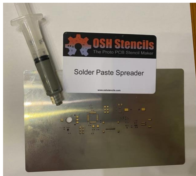
Figure 7. OSH Stencil overlaid on the circuit board, revealing the gold pads that require solder paste
