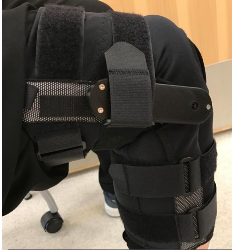
Figure 27b. The device (with the top and bottom of the casing employed) attached to the hinge system, which sits in the knee brace which is worn on a subject's leg
