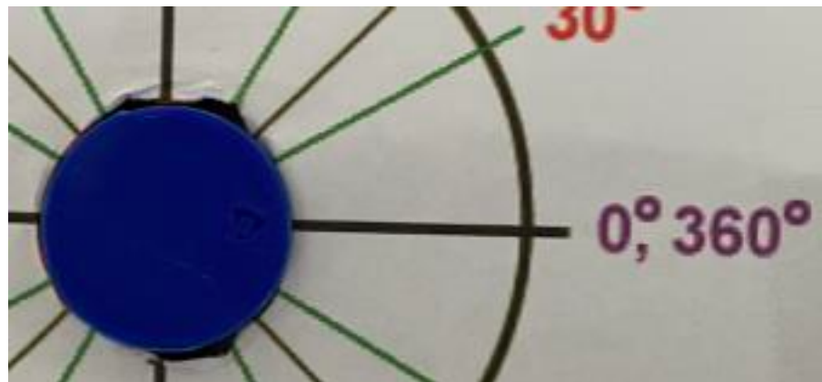
Figure 21. Close up of the unit circle overlaid on the case with the rotor shaft in place with the arrow at zero degrees.
