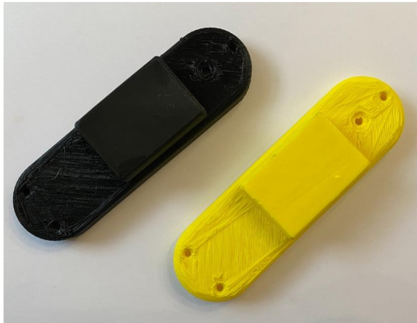
Figure 19. Printed Encasements with Uneven Print Job
